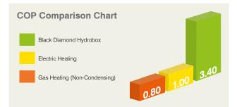
Heat pumps use electrical energy and take low grade heat energy from the outdoor air, to heat refrigerant which in turn heats water for domestic use. The efficiency of a heat pump is known as the Coefficient of Performance or COP. This is a ratio of the heat delivered to power consumed. For every 1kW of electrical input energy, the heat pump absorbs renewable heat energy from the outdoor air to provide the home with an average of at least 3.4kW\*<sup>2</sup> of heat output.
